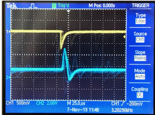
Figure 3.3: Signals visualization in the oscilloscope (up: preamplified signal, down: amplified signal)
