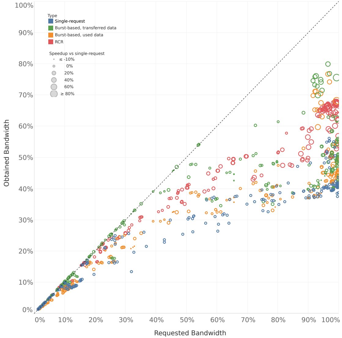
Figure 5.6 – Fraction of requested and obtained DRAM bandwidth during the execution of all benchmarks on all configurations, color-coded by MOMS architecture. The circle size is proportional to the speedup with respect to the single-request MOMS. Backpressure from the DRAM controller, a symptom of row conflicts, severely limits the DRAM bandwidth available to the single-request MOMSes. Both bursts and RCRs provide their highest speedups to data points that need the largest bandwidth. Burst MOMSes have higher bandwidth utilization but waste part of it internally. RCRs increase bandwidth utilization without incurring in data wastage and outperform the burst MOMSes on most data points in terms of bandwidth actually used.
