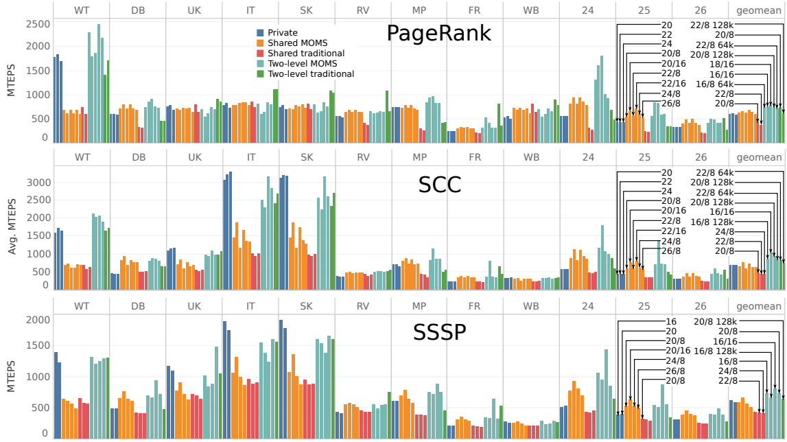
Figure 7.8 – Throughput on PageRank, SCC, and SSSP for different architectures. For shared and two-level architectures, the label X/Y Zk indicates X PEs and Y MOMS banks with Z kB of private cache. The two-level architectures with 16 banks generally provide the highest performance, balancing PE peak throughput, amount of conflicts in the shared MOMS, memory efficiency, and routing congestion.
