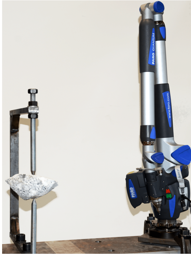
Figure 13: The laser scanner setup using the Quantum FARO Arm ® ; the left side of the picture shows the laser scanner used to scan the stone, and the right side shows the stone pinned on a steel frame for the scan to minimise the loss of surface data.
