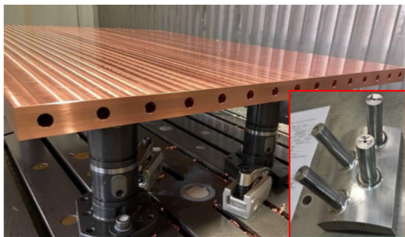
Fig. 11: Prototypes for qualification of deep drilling for ERID panel and extrusion/welding for Calorimeter manifolds
