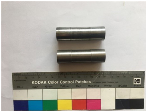
Fig. 5 On top: original engine's piston pin; at the bottom: new piston pin manufactured with a smaller diameter in the center, where the connecting rod is located ©MNAM 2019
