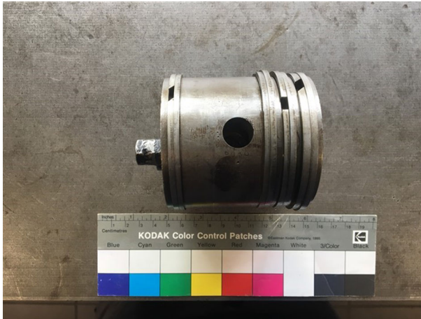
Fig. 6 Piston n.1 that has then been modified to simulate the wear of the rings ©MNAM 2019
