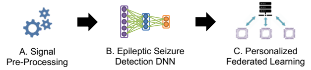
Fig. 1: Pipeline of the proposed FL process for epileptic seizure detection.
