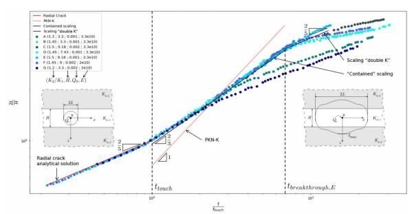
In the three layers set up, the analytical solution fits well before the propagation reaches the new media. After, the scaling developed is coherent with the propagation.
