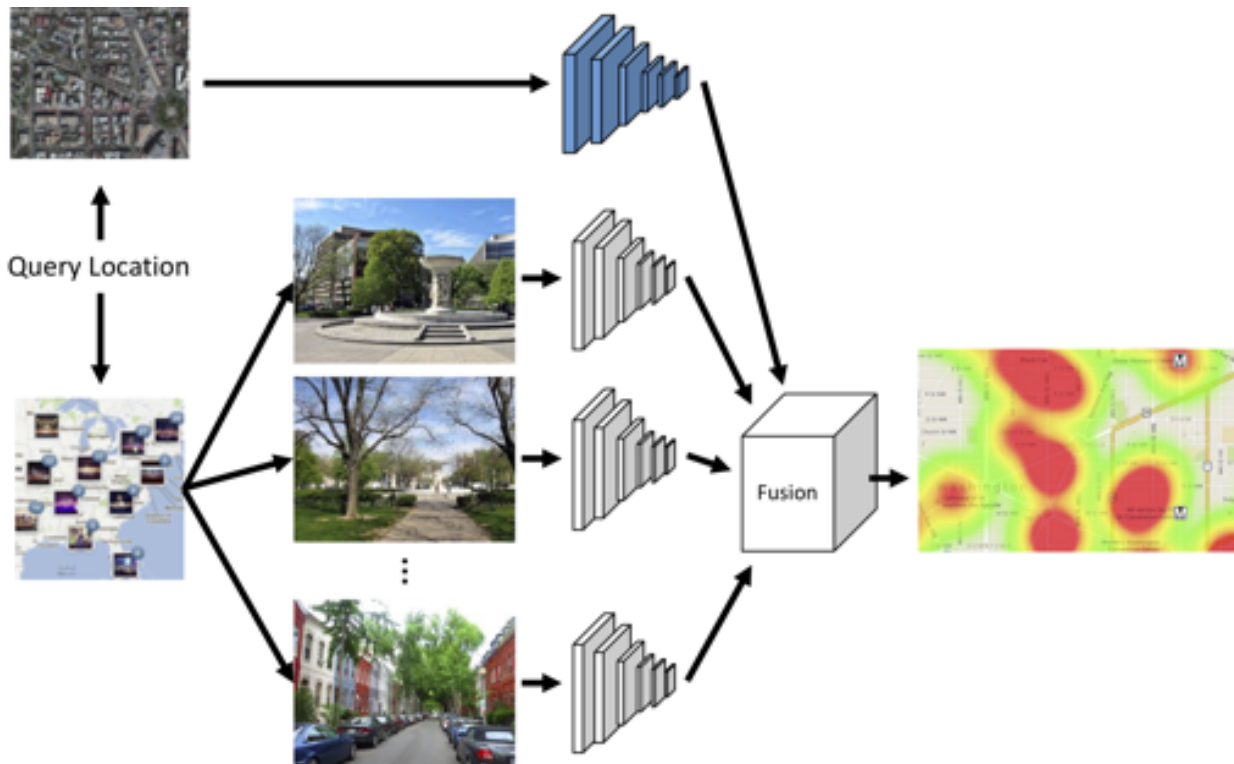
Fig. 2. Example of a system providing likelihood of presence of an object with multiple modalities. Ground and satellite images provide hard and weak (picture-based) labels respectively to create a heatmap of the presence of objects in urban areas. Location information is used to perform the fusion.
