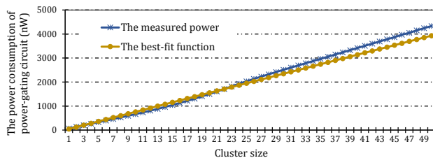
FIGURE 8. In blue, the power consumption of the power-gating circuit when the cluster is powered off, in the function of cluster size. We can notice that increasing the cluster size results in higher power consumption of the power-gating circuit. In yellow, the best-fit linear approximation.
