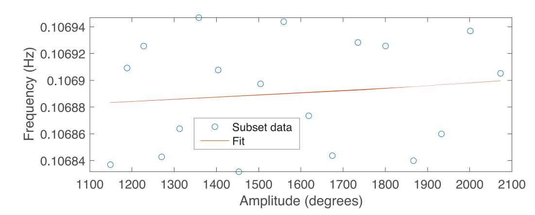
The nonlinear stiffness coefficients were derived from the coefficients of a second order even polynomial fit of the frequency-amplitude characteristic:  $\omega(\Theta) = \omega_0 + \omega^2 \Theta^2$ , yielding the nonlinear restoring torque
