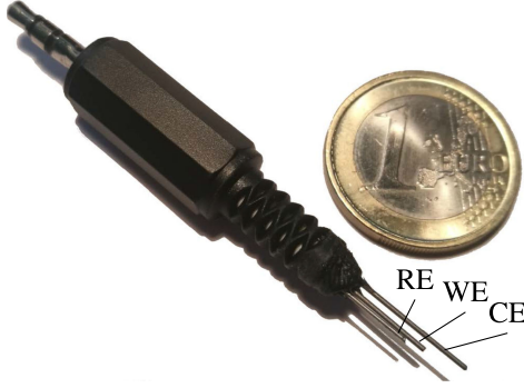
Fig. 4. Disposable pencil graphite needle-shaped sensor for detection of propofol in human serum.
