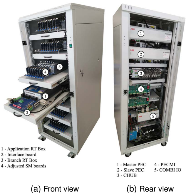
Fig. 7: HIL system used for model verification purposes.
