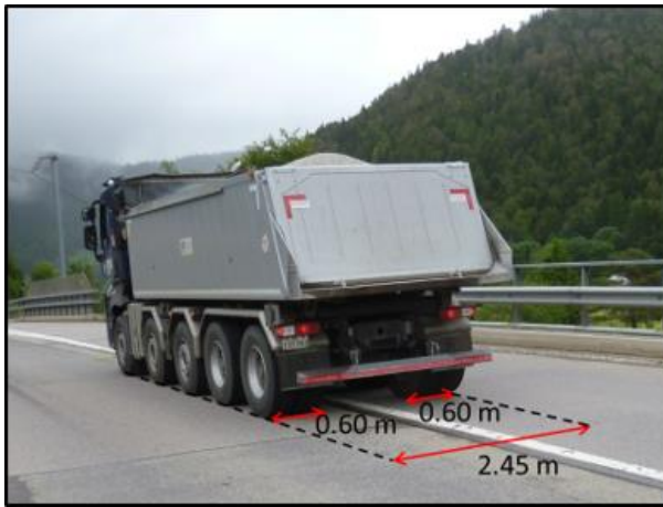
Load test, with a truck of five axles having the legal limit load of 400 kN.
