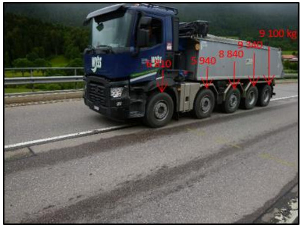
Load test, with a truck of five axles having the legal limit load of 400 kN.
