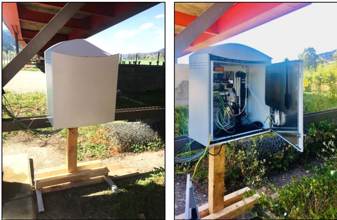
The made box for protecting the acquisition systems provided with a monitor for real-time visualisation of measurements.
