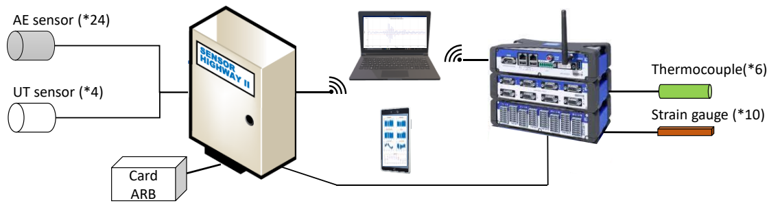
Figure 3.3. Configuration of the monitoring system.
