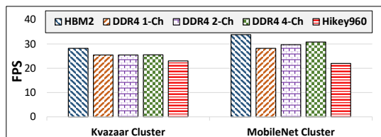
Fig. 18. Video Analytics FPS for Kvazaar and Mobilenet clusters for 300x200 resolution video for drone navigation when using HBM2, DDR4 and on Hikey960 platform.
