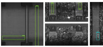
The evaluation is done on the test set on a total of 2279 images, with a total of 275 cracks and 406 flakings. The metrics used to assess the performance for each class are precision and recall, using a score threshold of 0,5 and an IoU threshold of 0,2.
