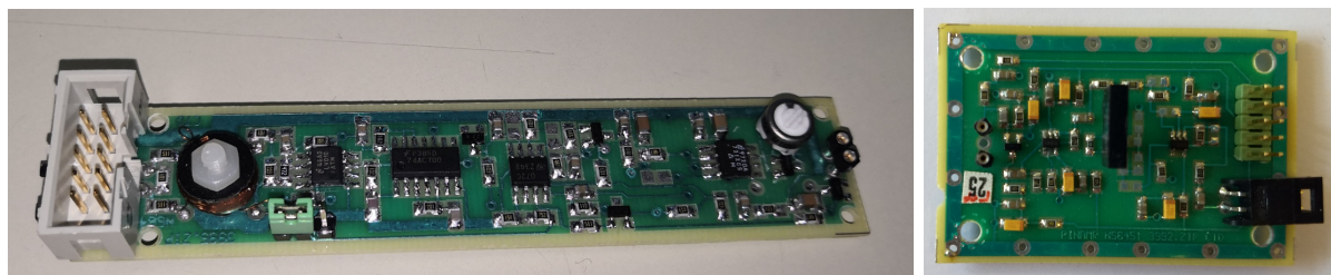
Figure 19: (Left) LHCb ECAL LED driver and (right) PIN amplifier, as used for PLUME.
