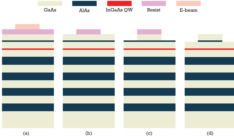
FIGURE 4.5: Scheme of the fabrication process. The MBE grown half-cavity: the bottom DBR and the \lambda -spacer layer with a single QW, with the e-beam resist on top. (a) e-beam resist deposition and e-beam exposure of the patterns. (b) developing the e-beam resist (c) wet etching (d) removing the AlAs etch-stop and e-beam resist layers.
