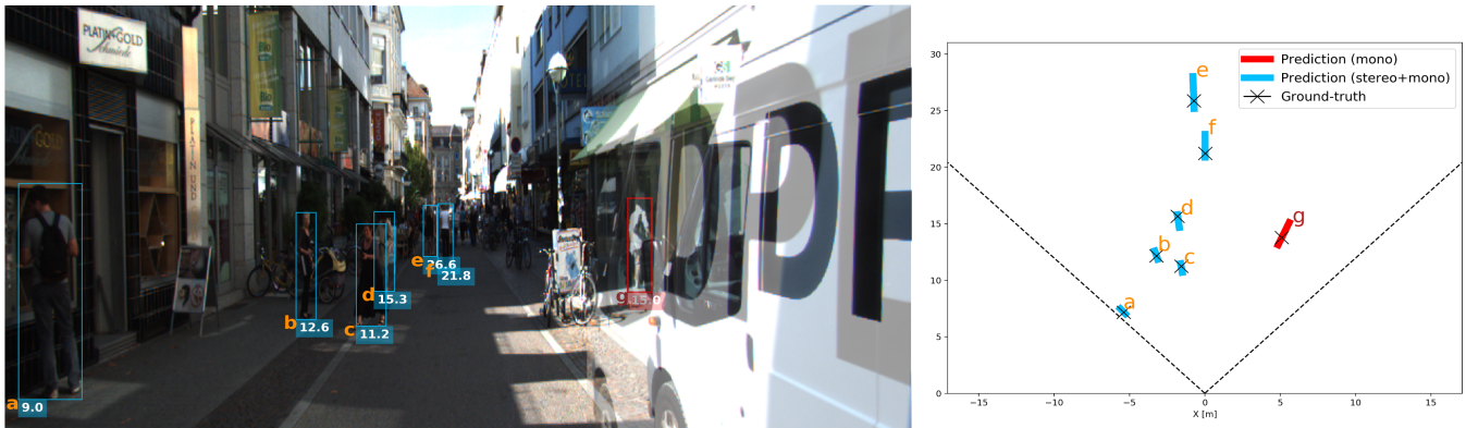
Fig. 1: Long tail example in the KITTI dataset [6]. The pedestrian g is only visible from the left camera (no stereo information available) as shown by overlapping the white van from the right image. The network classifies it as a monocular sample (red color) and outputs a larger confidence interval that reflects less accurate monocular estimates at that location. We display radial distances in meters in the frontal image and radial uncertainties in the bird-eye-view image. Only instances that match a ground-truth are shown.
