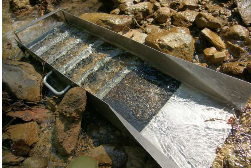
Figure 8: Sluice for gold washing. Mud is transported to the sluice to be washed. Gold nuggets and particles will deposit at the bottom because of its density and can be retrieved without further processes. Illustration from Wikimedia Commons 45
