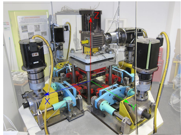
Fig. 9 The BCR-3D shear device with the three principal loading axes X , Y and Z (Stavropoulou et al. 2019)
