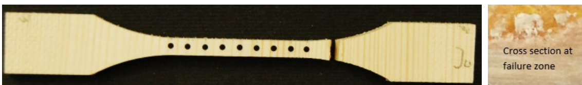
Fig. 22. Specimen TT-032-02-REB3 with a resin check.
