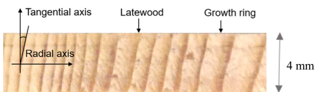
Fig. 5. Change of the angle between the local tangential and radial directions, and latewood and growth ring thickness change.
