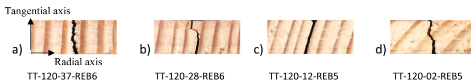
Fig. 17. Different failure modes observed in specimens: a) Earlywood failure, b) Earlywood-border failure, c) Growth ring border failure, d) Crossing growth ring failure. Vertical dimension is 4 mm (specimen width). Load is applied along the radial axis.
