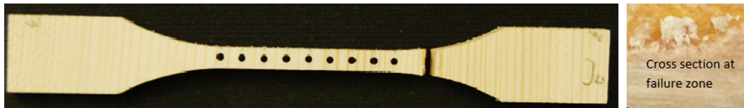
Fig. 22. Specimen TT-032-02-REB3 with a resin check.
