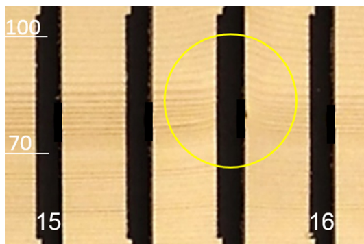
Fig. 19. Area affected by a small knot in REB5 (two cut specimens between specimens 15 and 16 were unusable and excluded).
