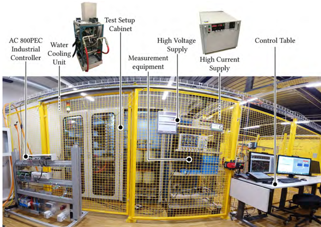
▲ IGCT characterization test setup
