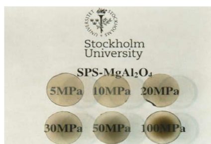
Figure 1. The 12 mm diameter magnesium spinel samples demonstrating sintering inhomogeneities occurring during spark plasma sintering (SPS). Direct observation of the inhomogeneities is possible due to the observed optical differences, accentuated with increasing uniaxial pressure applied during the heating ramp prior to reaching the final dwell temperature (1300 °C for 3 min). The brownish-black discoloration is believed to be directly linked to dislocation stabilized oxygen vacancies, likely to be generated as a result of superplastic deformation occurring at low temperature [47]. (reprinted with permission from Elsevier).
