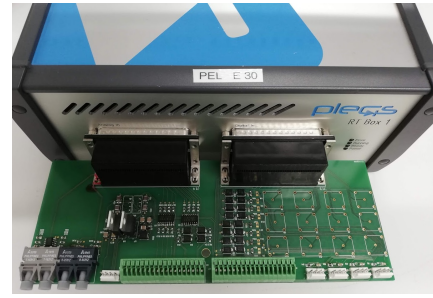
Fig. 5: A PLEXIM RT-Box fast control prototyping platform is fitted with a custom interface board to control the SSBTS prototype for the purpose of the laboratory testing.
