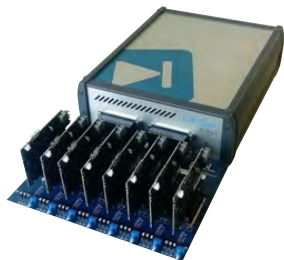
▲ RT Box hosting eight MMC sub-modules
