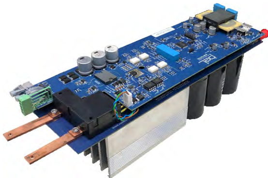
▲ Developed MMC FB sub-module based on the 12kV IGBTs
