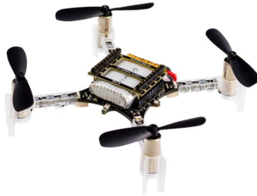
Figure 1: Crazyflie 2.0 nano quadcopter
