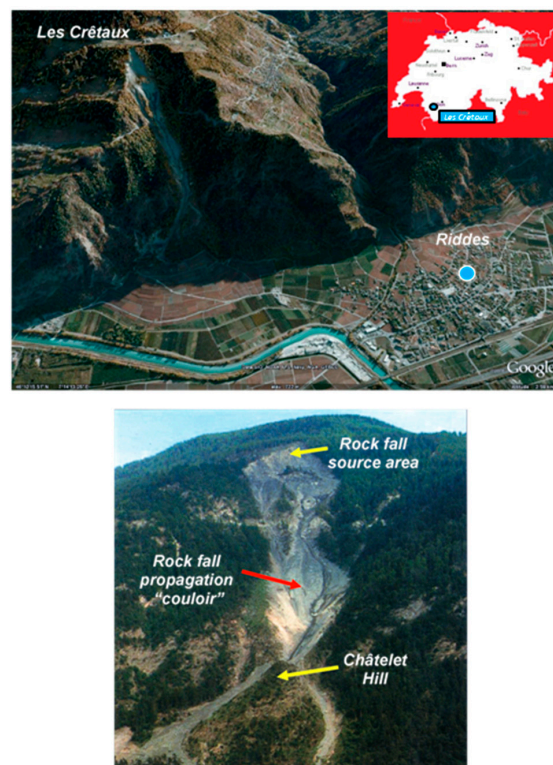
Figure 11. Area of Les Crêtaux, Canton of Valais (Switzerland). Top: location and aerial view of the study site (sources: www.petiteviree.com , Google Earth). Bottom: front view of the rock fall source area and the corridor located just below (source: [17]).
