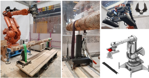
Figure 20: Robotic fabrication and scanning setup employed to cut both straight, curved and forked beams using 2-rail system and Faro S150 laser scanner fixed to the gripper.
