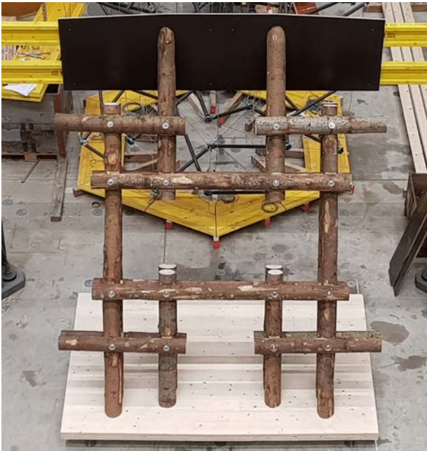
Figure 22: Prototype of a two-layer reciprocal system.
