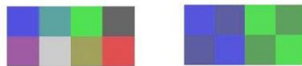
Figure 4: Left: a schematic view of 4 : 4 : 4 method. Right: A schematic view of 4 : 2 : 0 method that benefits from chroma subsampling [19][20].
