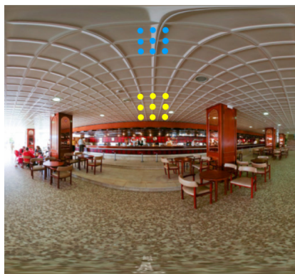
Figure 10: Implementation of planar 3 \times 3 kernel on an omnidirectional image from SUN360[16] dataset. The main problem happens when the kernel is applied on the lower parts or upper parts of the image.
