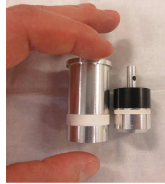
Fig. 5. Linear self-shielded reactivity modulator in ZED-2 reactor: a piston (right) and sleeve (left) coupling [15].
