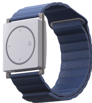
Figure 13. Embrace2 by Empatica Inc. [72] for seizure detection (Image reprinted with kind permission of Empatica Inc.).
