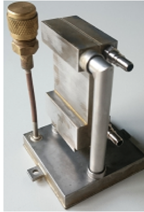
Figure 2.2 – Thermosyphon prototype designed and manufactured by Seuret et al. [20]
