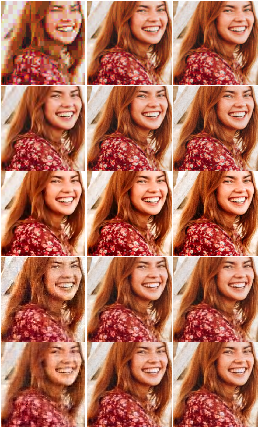
Figure 7.6 – Reference image in Figure 7.3c compressed using JPEG, JPEG 2000, WebP, ResWCAE and ResMixWCAE from top to bottom, at target bitrates 0.12, 0.50 and 1.00 bpp from left to right, respectively.
