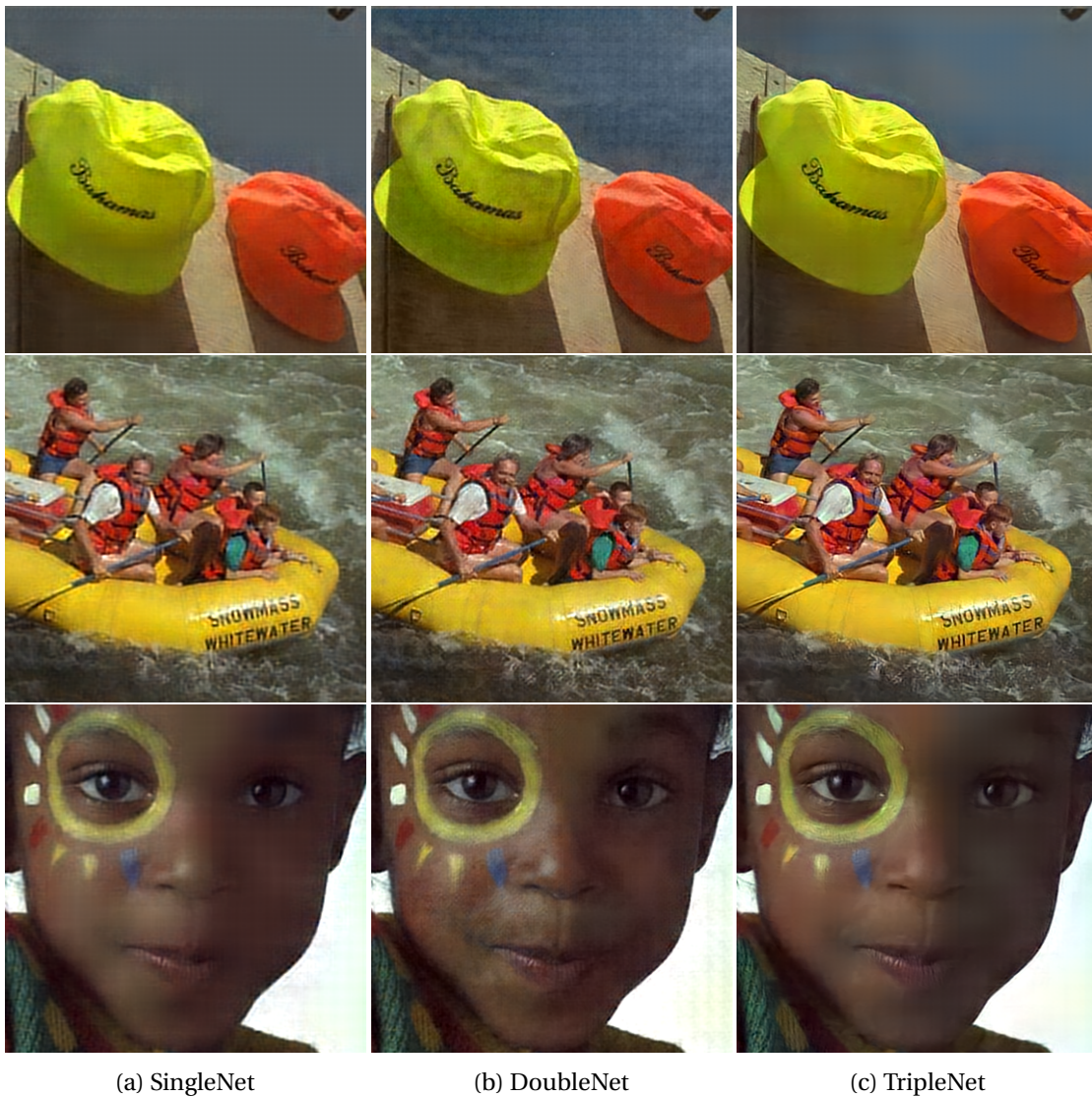
Figure 8.4 – Cropped sections of kodim03, kodim14 and kodim15 images from Kodak image database, compressed before cropping using SingleNet, DoubleNet and TripleNet at target bitrate 0.50bpp.
