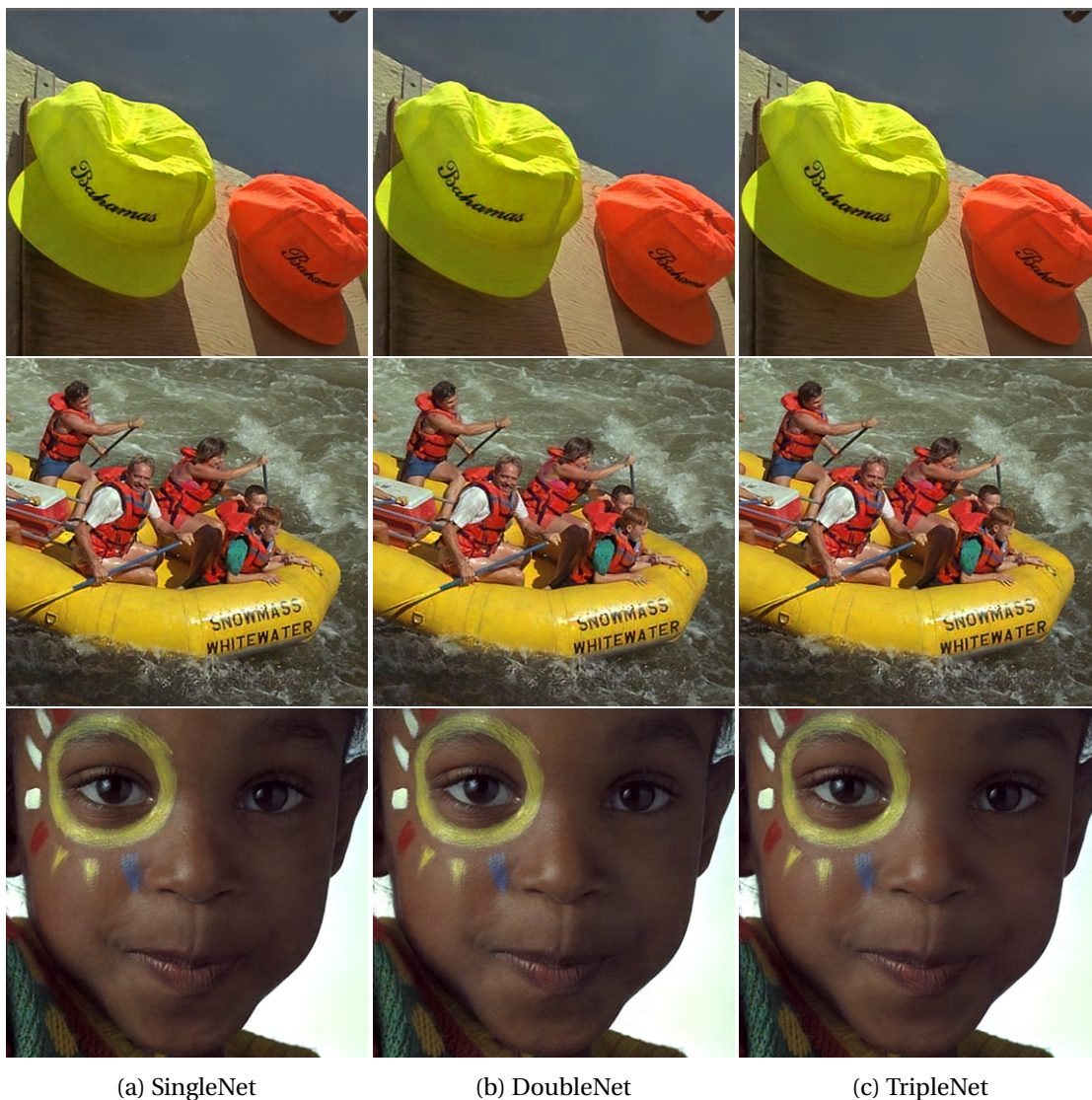
Figure 8.6 – Cropped sections of kodim03, kodim14 and kodim15 images from Kodak image database, compressed before cropping using SingleNet, DoubleNet and TripleNet at target bitrate 1.00bpp.
