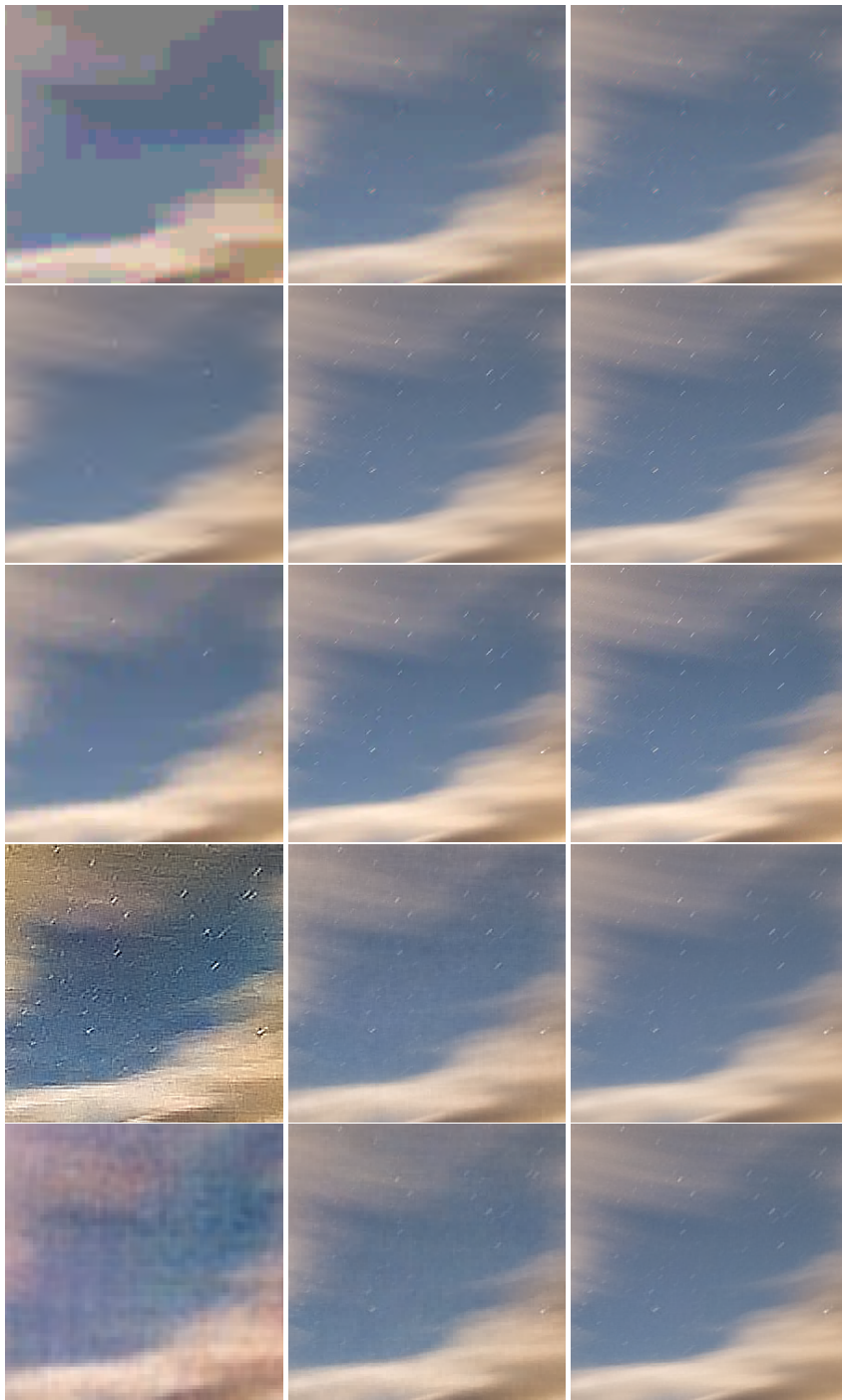
Figure 7.4 – Reference image in Figure 7.3a compressed using JPEG, JPEG 2000, WebP, ResWCAE and ResMixWCAE from top to bottom, at target bitrates 0.12, 0.50 and 1.00 bpp from left to right, respectively.
