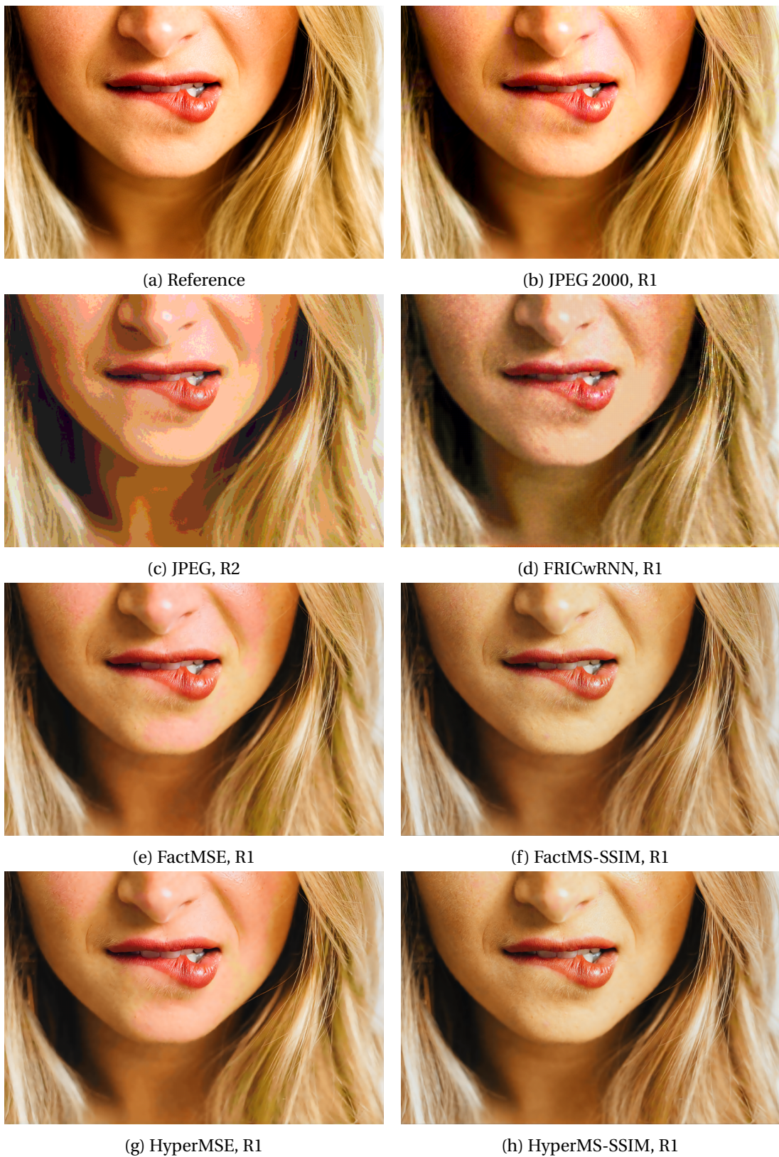
Figure 4.18 – Test content TE08 compressed at target bitrate 0.06bpp, using JPEG 2000, JPEG, FRICwRNN, FactMSE, FactMS-SSIM, HyperMSE and HyperMS-SSIM.
