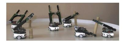
Fig. 1. Physical set-up for the stick pulling experiment.
