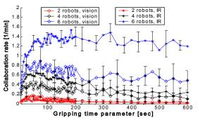
Figure 8: For a scan interval of 30 cm and scan angle of 360°, the advantage of the larger field of view of the IR team is apparent.
