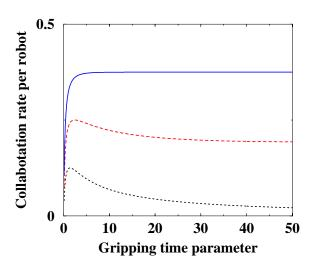
Figure 8: Collaboration rate per robot vs (dimensionless) gripping time parameter  $\tau$  for  $\beta=0.5$  (short dash),  $\beta=1$  (long dash),  $\beta=1.5$  (solid line). These values of  $\beta$  correspond, respectively, to two, four, and six robots in the experiments with four sticks (cf. Fig. 5).
