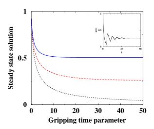
Figure 7: Steady state solution vs (dimensionless) gripping time parameter  $\tau$ : for  $\beta=0.5$  (short dash), 1 (long dash), 1.5 (solid line). Inset shows a typical relaxation to the steady state for  $\tau=5,\,\beta=0.5$ .
