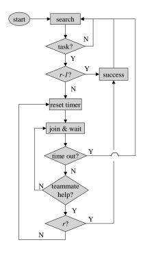
Figure 1: Schematic of a robot's controller for collaborative task completion.
