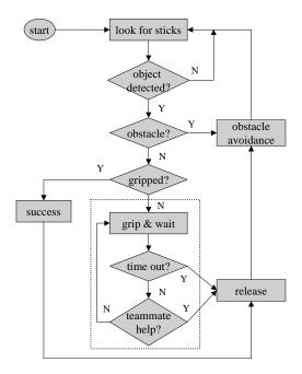
Figure 4: Flowchart of the robots' controller reported from [14] with overlapped state blocks.
