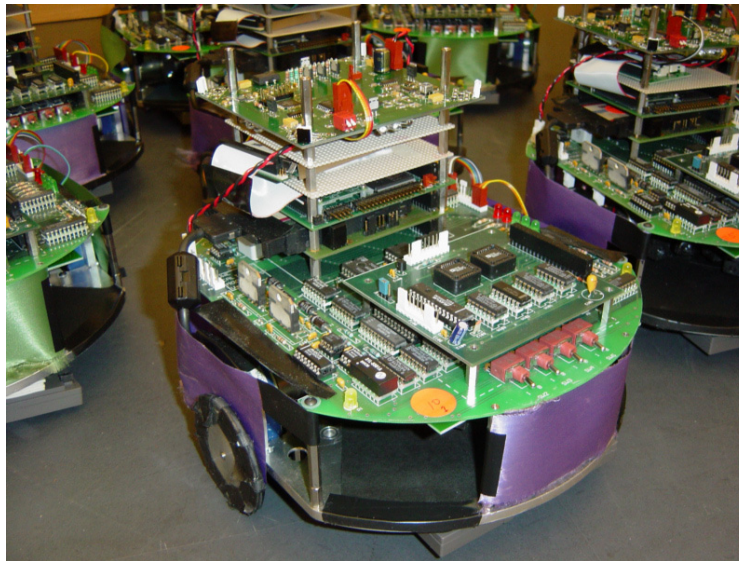
Figure 2: Close-up of a Mooreboot with the localisation and communication board (board on top of the PC104 stack on the back of the robot).
