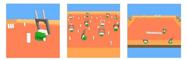
Figure 1 *Left*: close-up of a simulated robot equipped with a gripper, ready to grip a seed. *Center*: corresponding setup in the embodied simulator (10 robots, 20 seeds, 178 x 178 cm<sup>2</sup> arena). The inner area represents the working zone and the surrounding area is the parking/resting zone where robots that decide to stop working stay idle. *Right*: typical end of aggregation experiment, e.g., 5 hours of simulated time, in a 178 x 178 cm<sup>2</sup> arena.
