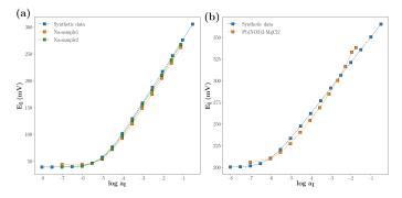
Fig. 3: Fitting synthetic and measured calibration curves: (a) sodium sensor calibration, (b) lead sensor calibration with magnesium as interferent ion.
