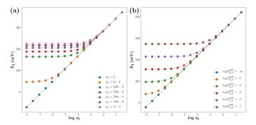
Fig. 2: Parametric analysis of multi-ion sensing: (a)  $a_J$  swept from 0 to 1e - 3, with  $z_I = 1$ , offset = 400 mV,  $z_J = 1$ , and log  $K_{I,J}^{pot} = -3$ ; (b) log  $K_{I,J}^{pot}$  swept from  $-\infty$  to -1, with  $z_I = 1$ , offset = 450 mV,  $z_J = 1$ , and  $a_J = 10e - 6$ .
