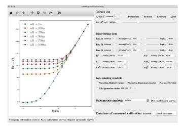
Fig. 1: GUI developed to generate synthetic calibration curves in different mixed-ion solutions, to perform parametric simulations, and to compare synthetic curves with database of in-vitro calibration curves.
