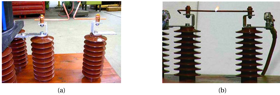
Figure 4.15 – Two types of fault emulators with spark gaps used in the pilot test. (a) A 14-cm long spark gap for the single-arcing fault and (b) a 3.5-mm long spark gap for the intermittent-arcing fault.
