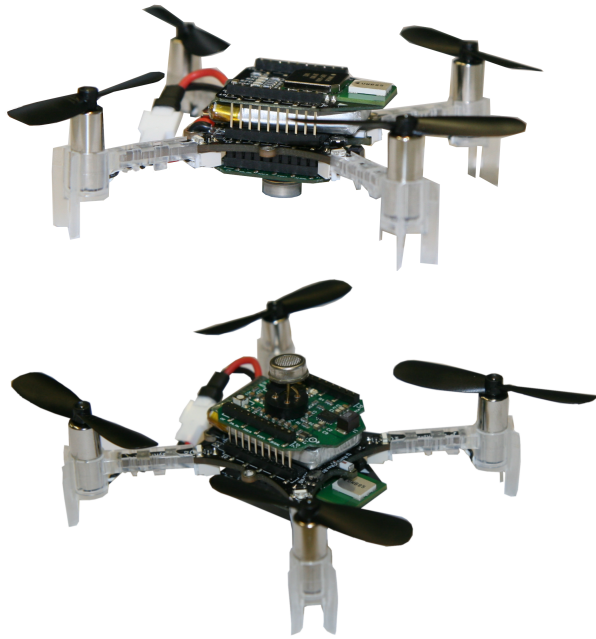
Fig. 1. Crazyflie V2.1 equipped with a custom PCB for odor sensing. Both sensor configuration (top and bottom) are presented.
