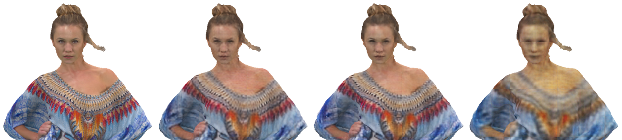
(a) Reference (b) 1:1, \lambda_g = 2500, \lambda_c = 2500 (c) 1:19, \lambda_g = 250, \lambda_c = 4750 (d) 19:1, \lambda_g = 4750, \lambda_c = 250 Figure 8: Visual comparison for content longdress, for different distortion allocation ratios.
