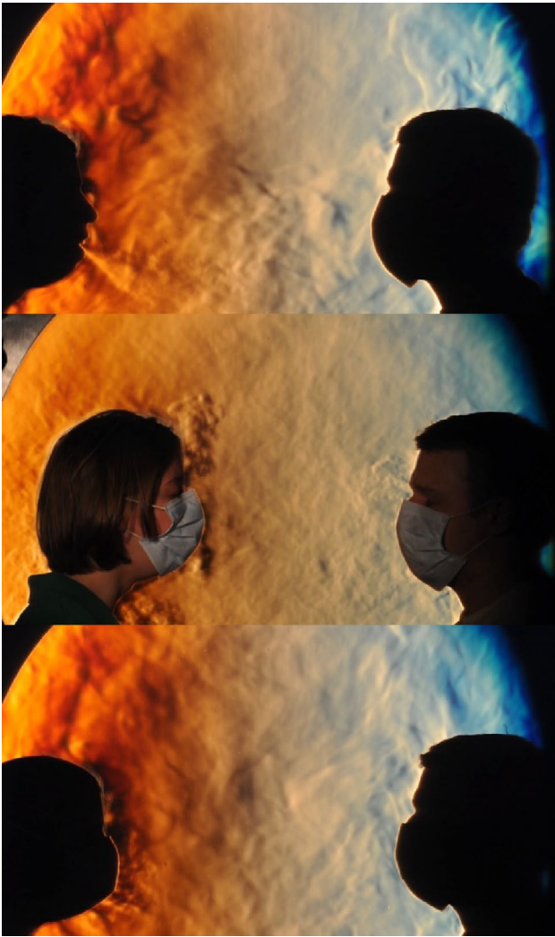
Fig. 22 Schlieren images of two volunteers. The roughness of the Schlieren image is related to the turbulence of the emission, and visualizes the fluid flow of the emitted aerosols. In one instance, a person coughs without any mask protection (top), wearing a surgical mask (middle) and finally a FFP2 mask (bottom). The flow direction is inclined 308^\circ downward in the top image. It has both vertical components (downward and upward) and lateral components that bypass the surgical mask in the middle image. The best fit of a FFP2 mask reduces the bypass flow but it increases the flux released through the mask. However, its weak speed limits the region affected by exhalations to the immediate neighborhood of the volunteer (images provided by Gary S. Settles)
