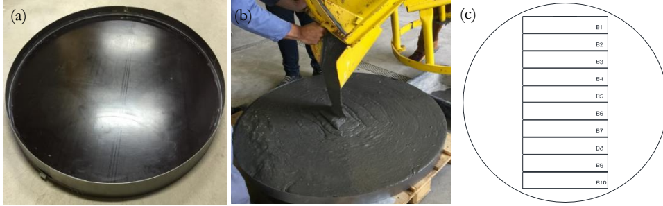
Figure 2 Specimen preparation: (a) circular formwork; (b) casting method; (c) extracted plates for 4PBT
