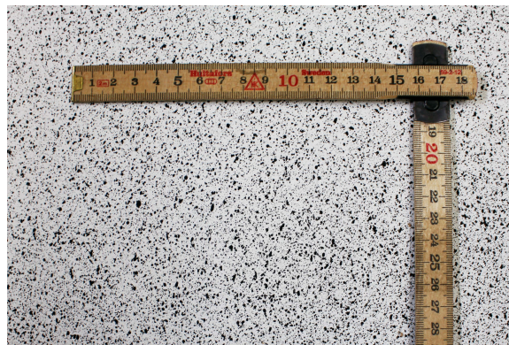
Figure 3.6 – Speckle pattern used for the DIC data acquisition. Speckle sizes between 1 and 5 mm were obtained by applying black paint on two coats of matte white paint with a pneumatic paint sprayer.
