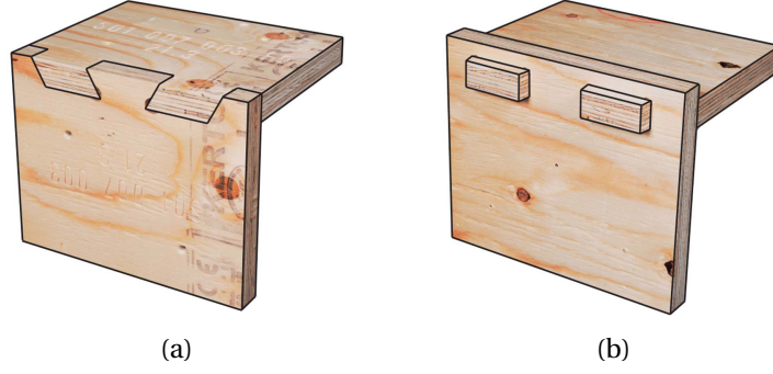
Figure 1.4 – Single-degree-of-freedom (1-DOF) multiple tab-and-slot joints (MTSJ): (a) Open-slot and (b) Closed-slot (MTSJ-TT). Reproduced from [104].
