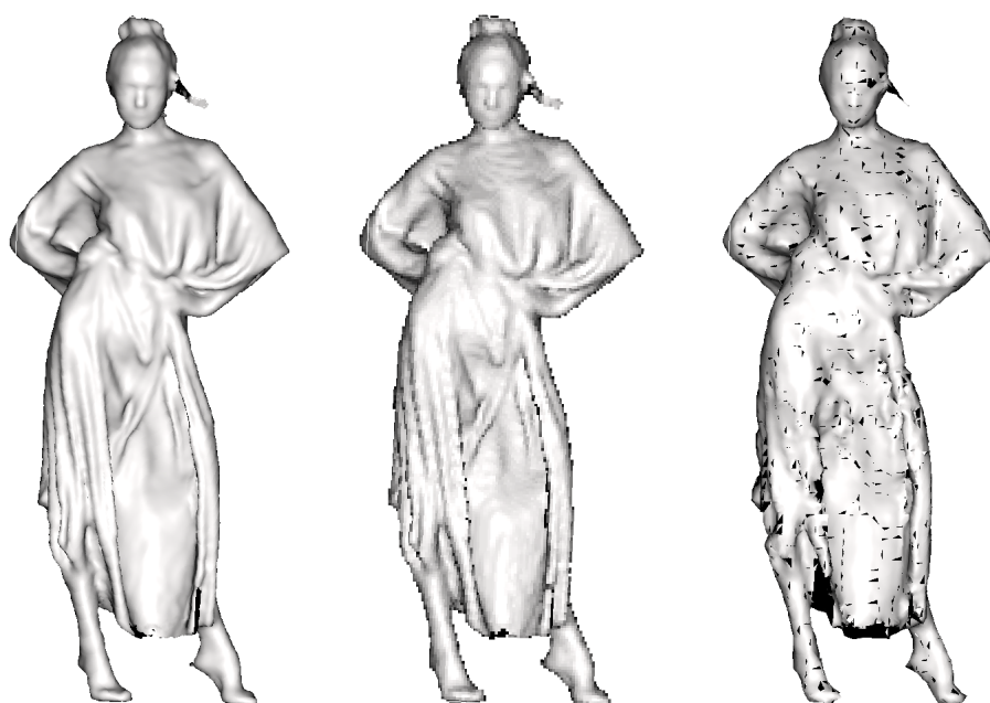
Figure 10: Three versions of the longdress model: reference, stimulus after encoding with Octree at R02, and stimulus after encoding with TriSoup at R01 following the MPEG CTC [12], from left to right. The normal vectors are estimated using plane fitting with range search and radius 10. The obtained plane-to-plane similarity scores are 0.8830 and 0.7958, for the second and third stimulus, respectively.
