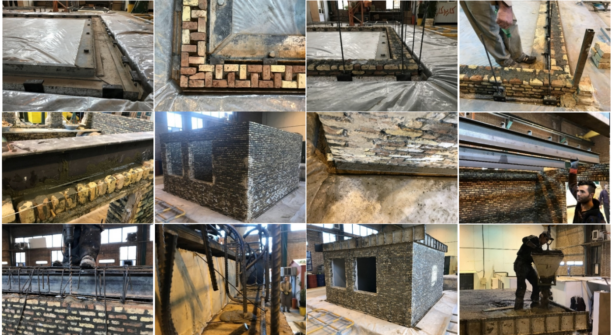
Figure 6. URM specimen construction procedure
