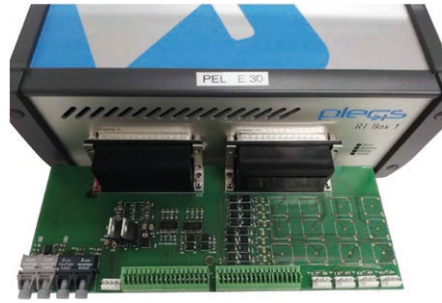
Fig. 9: PLEXIM RT Box with SSBTS interface board. The board provides the RT Box with fibre optical interface to the SSBTS gate driver, and electrical interface to the sensors. Additionally, analogue and digital I/Os are available for the controller to be externally accessed.
