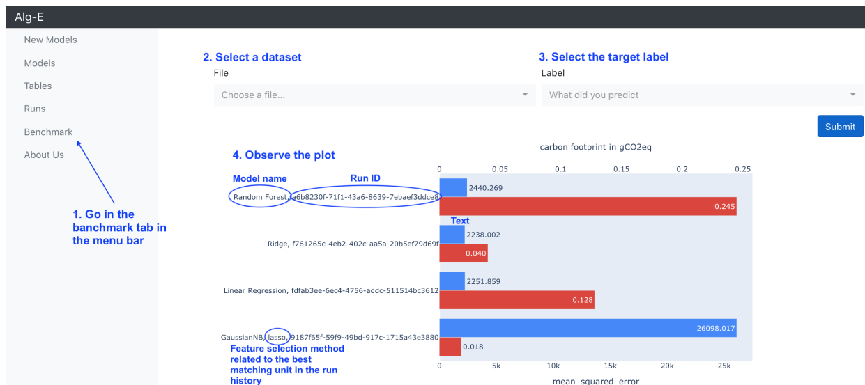
Figure 5.7: Chart displaying the highest accuracy within all runs of each model and the related carbon footprint and the steps to plot it
